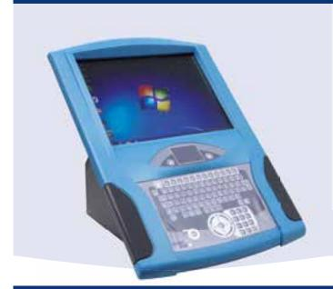
The Color Computer System EX is a Zone 2 approved computer that can be safely used in bodyshops and mixing rooms. The computer is dust-resistant and easy to clean. The hardware has been optimised for using ICRIS software. To ensure that you meet local legislative requirements, check in advance to see what zone approval is required in your country or region!
