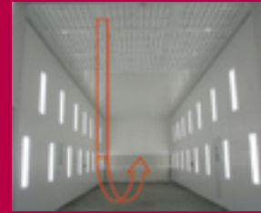
End draft spray booth, cross flow booth
