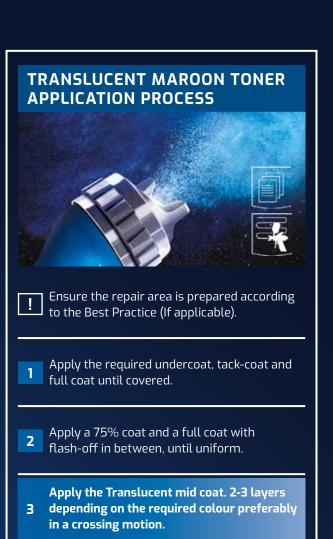
4 Apply a recommended clear coat suitable for the WaterBase 900<sup>+</sup> Series.
